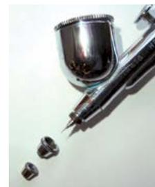
Figure 1: To stipple with the Iwata HP-C, remove the needle cap and nozzle cap (the two front-most pieces) from the airbrush. Be very careful not to drop the airbrush with these pieces removed.
